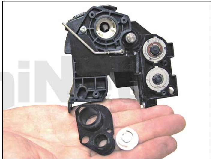
6. On the opposite side (non gear side) pry off the white gear and the drum bushing.
