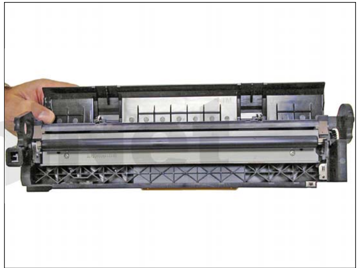
13. Clean the PCR with your normal cleaner. Wipe off the old conductive grease from the shaft and replace. Re-install the PCR in the assembly grease side to the black PCR holder.
