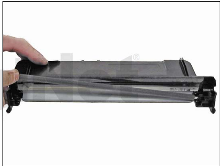
9. Remove the PCR cleaning roller. Clean the PCR with your normal PCR cleaner.
