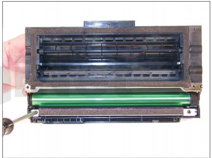
20. Install the PCR cleaner assembly.
