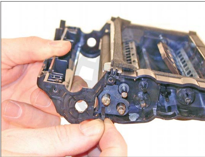
17. Install the roller plate.
