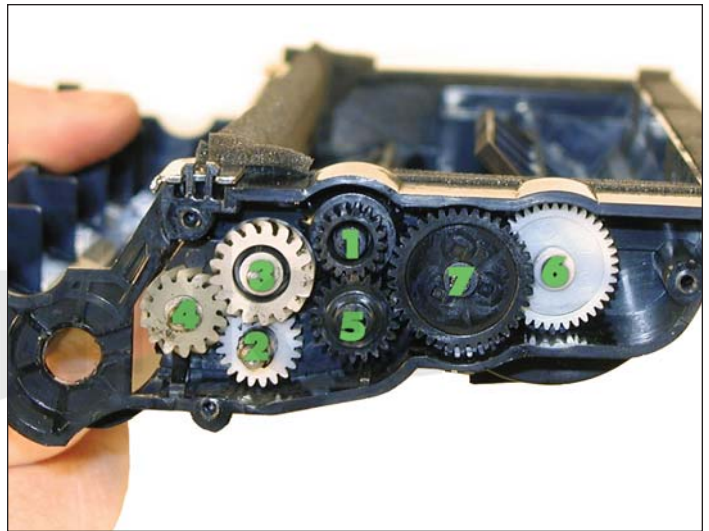
18. Replace the roller plate and seven gears. Look carefully at the picture of the gears. Each gear must fit in this exact way. The gears labeled in order of installation.
