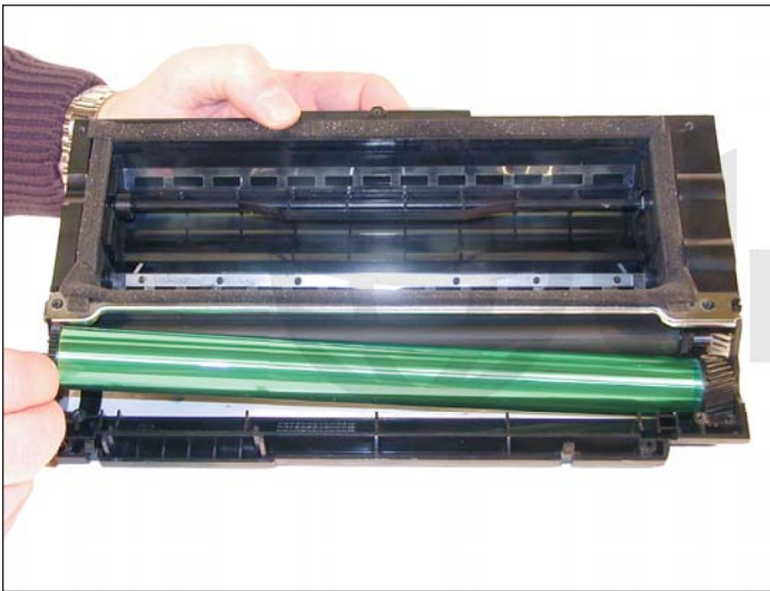
19. Install the new drum in place.
