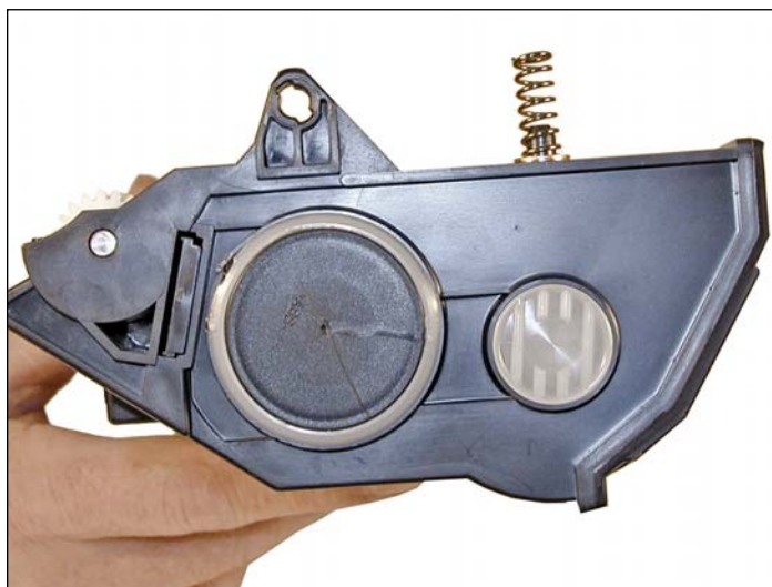
23. Install the fill plug, check for leaks. If the round chip fell off, just throw it away. A new chip will be installed later in the instruction.
