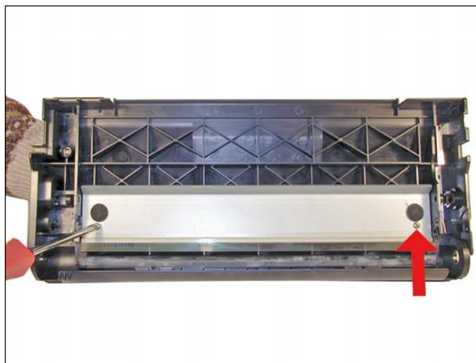
9. Coat the wiper blade with your preferred lubricant, and install in the cartridge. Install the two (gold) long screws, the four short screws are for the drum axle pins only.
