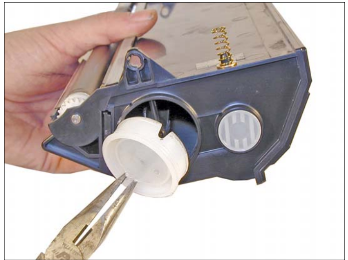
14. With the pair of needle nose pliers, pull the fill plug out. Grasp the plug by the small cross braces, and pull. This method does not damage the plug seal. Dump out any remaining toner from the hopper.
