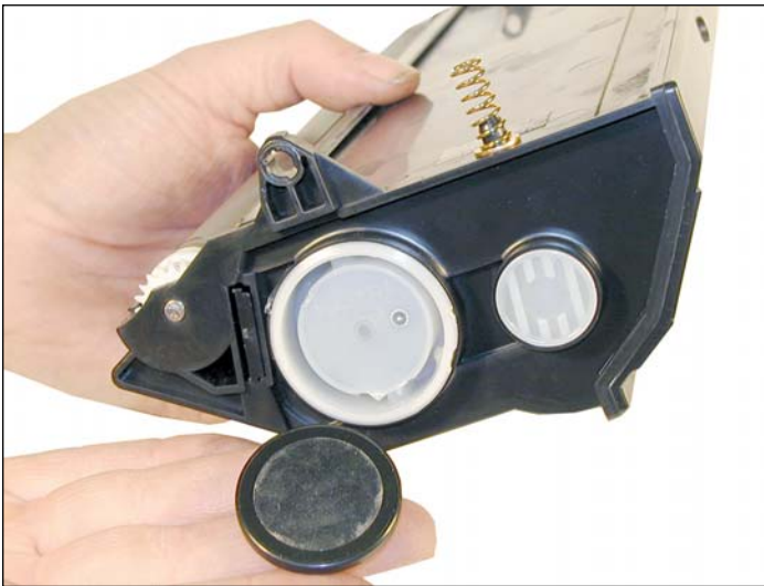
13. With a small jeweler's screwdriver, pry the black cover off the fill plug.
