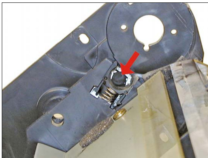
10. Clean the PCR contacts with a cotton swab and alcohol.
