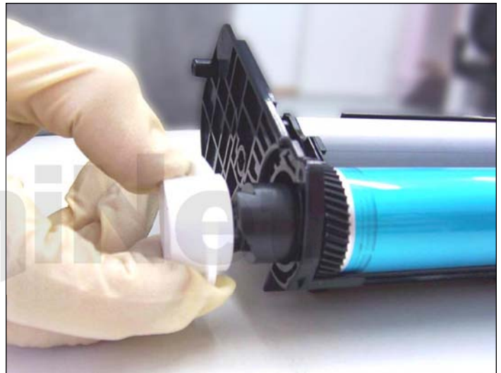
19. Remove the drum gear holder by pulling it out.
