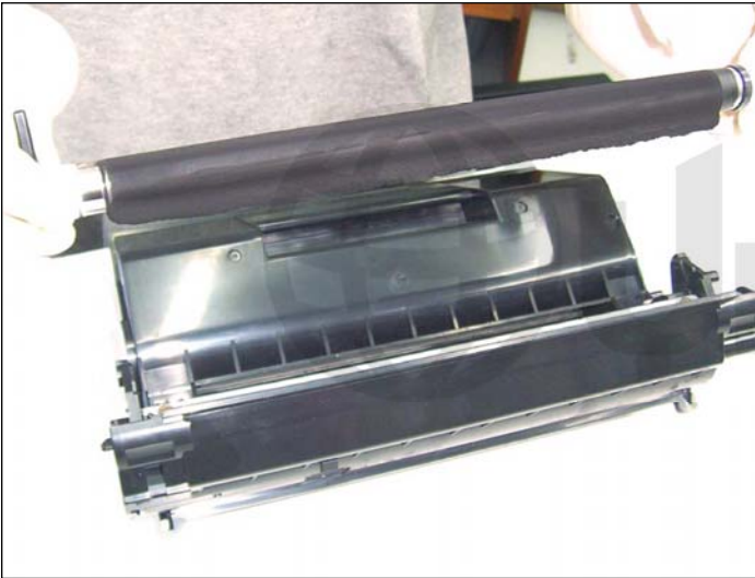
41. Continue with the other side until the magnetic roller is completely removed.
