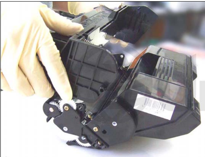
14. Lift evenly to separate the drum unit from the cartridge.
