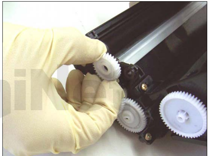
38. Remove all gears from the cartridge shown.
