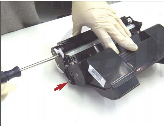
36. Remove the end-cap on the gear-side of the toner cartridge by first removing two gold-colored screws as shown.
