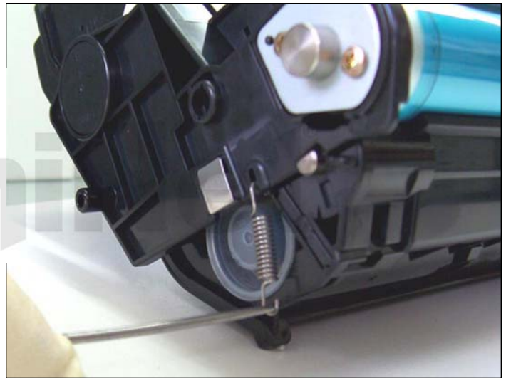
13. Use a hook tool to release the spring from the gearless side.
