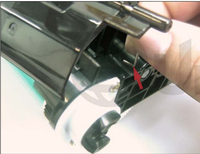
4. Remove the shutter door arm from the slot on the gear-side of the toner cartridge as shown.
