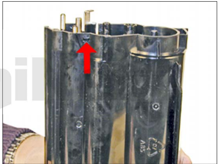
13. Install the small internal end cap.
