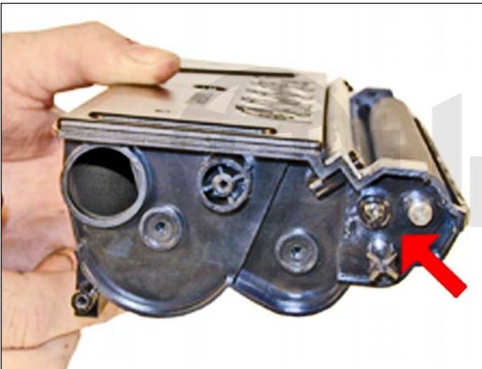
14. Install the developer roller end cap, screw, and drive gear on the waste chamber side. Clean the old grease off the gears and replace with new. We recommend white lithium grease be used.
