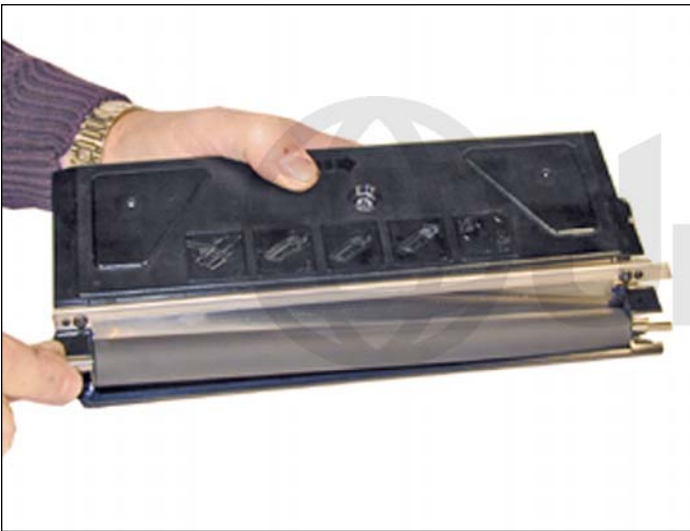
12. Install the developer roller.
