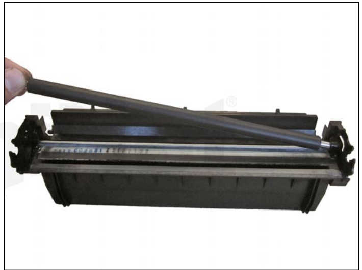
10. Remove the PCR from the assembly. Clean the PCR with your normal PCR cleaner.
