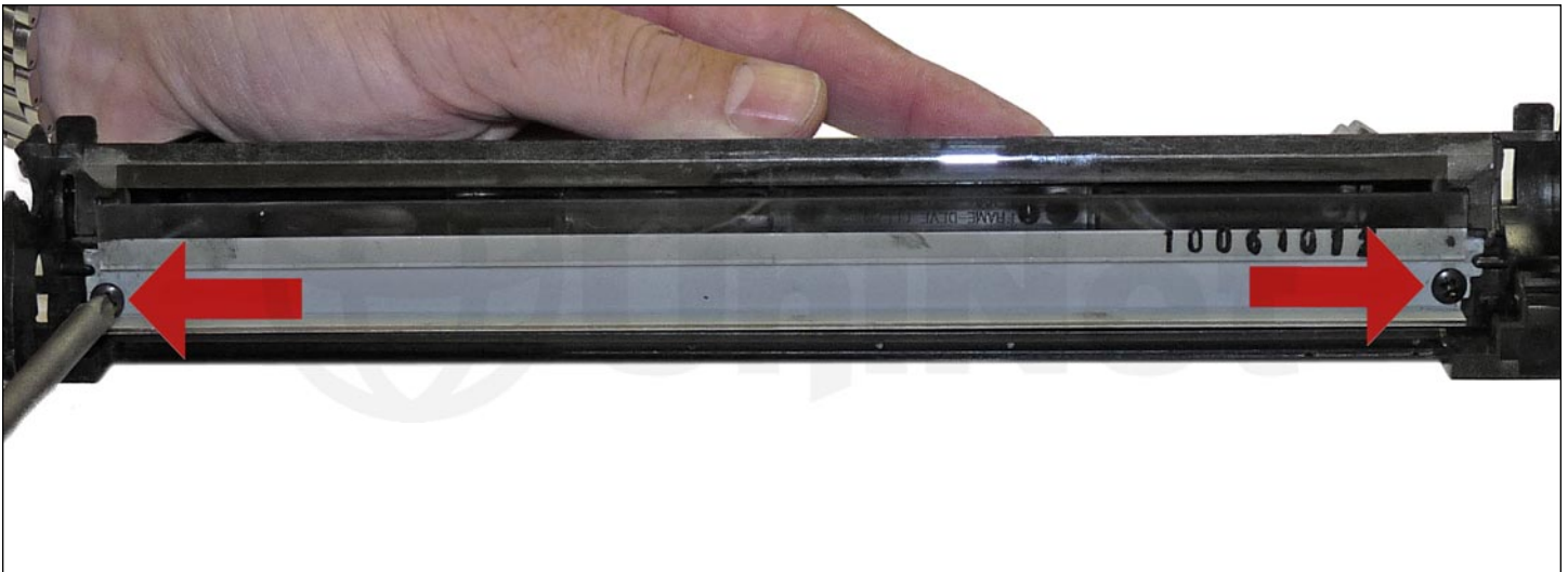
16. Install the cleaned (or new) wiper blade and two screws.
