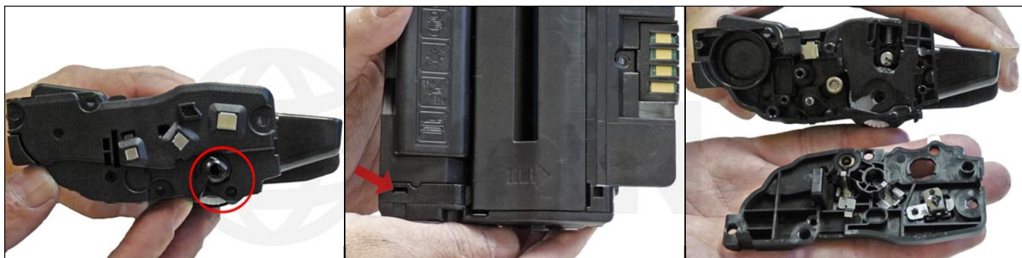
6. On the right side end cap: remove the remaining arm and press in on the top tab.
