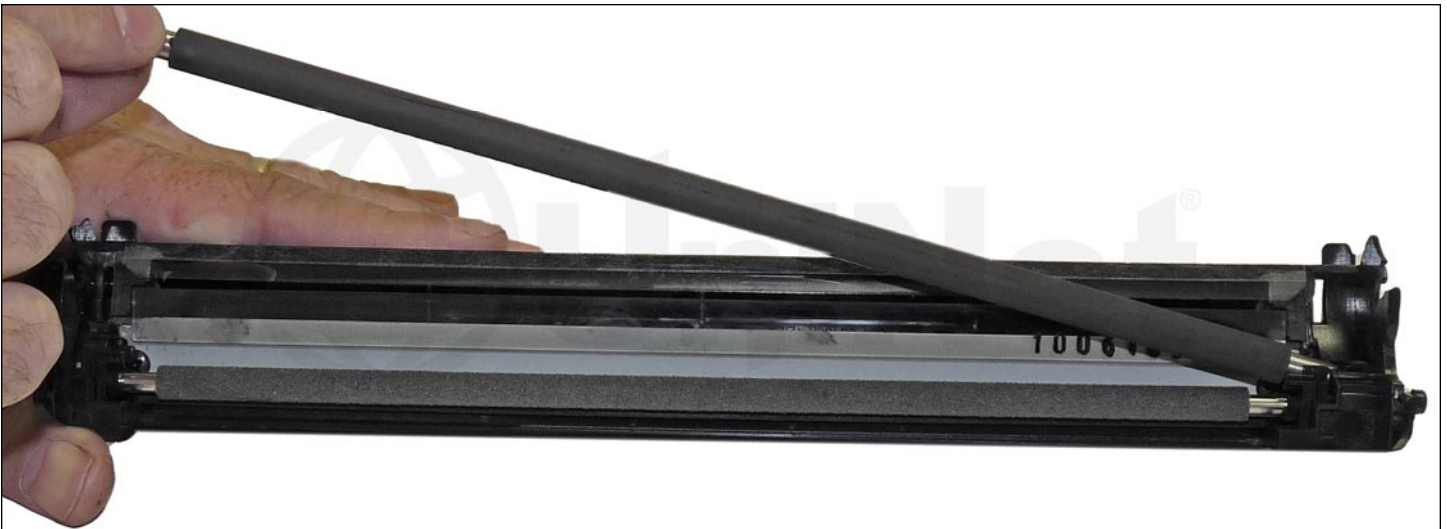
10. Remove the PCR (primary charge roller) from the assembly.
