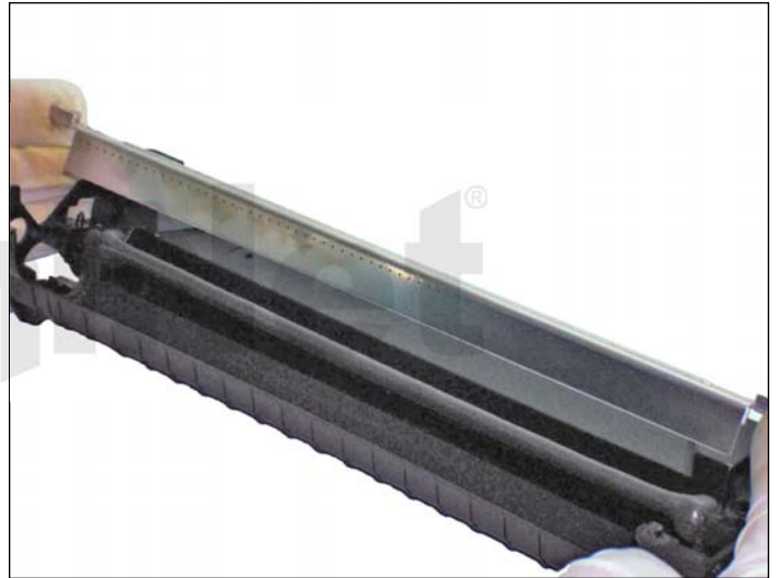
10. Unscrew and remove doctor blade.
