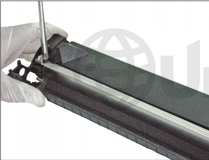
10. Unscrew and remove doctor blade.
