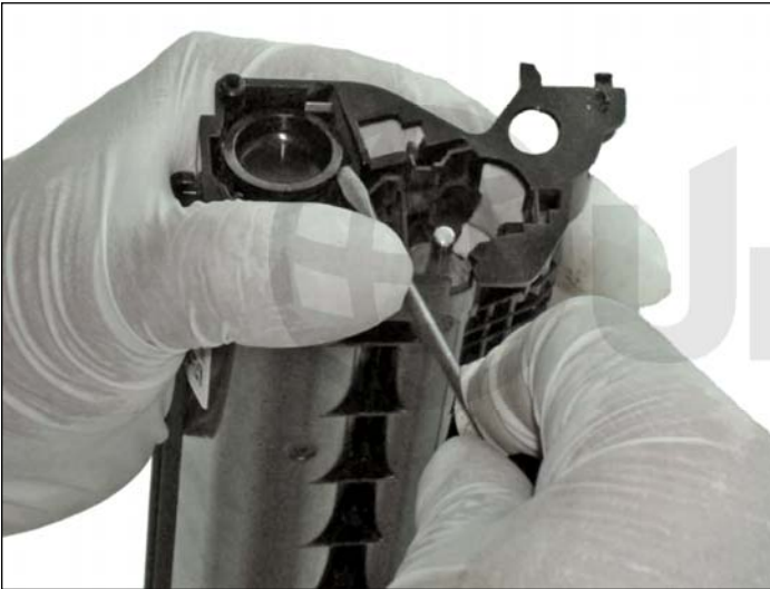
9. Remove the fill plug and vacuum the toner hopper clean.
