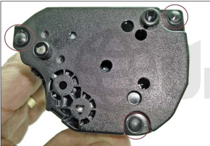
Side cover showing plastic rivets
