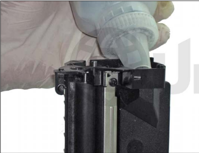
13. Fill the toner hopper with the proper amount of toner for use in Samsung ML-1665, and tightly close with the plastic lid.
