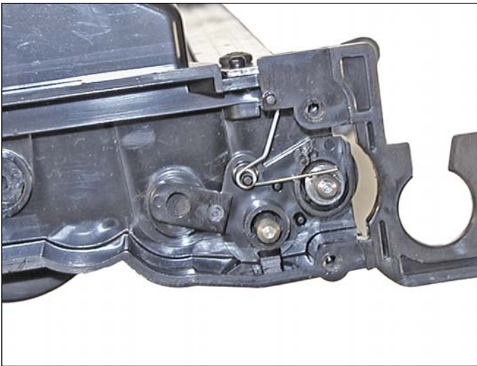
19. Snap the spring/plastic bushing assembly in place.
