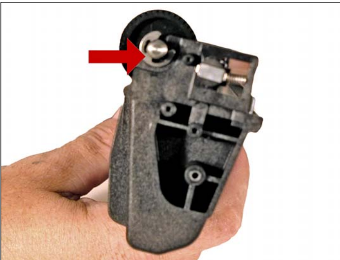
22. On the waste hopper, remove the E-ring from the drum axle.
