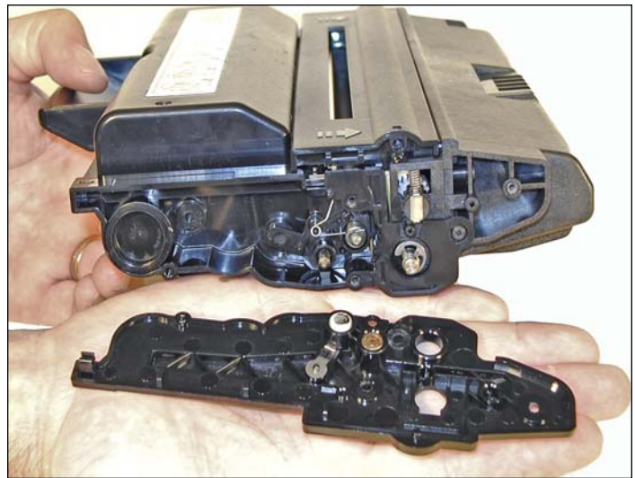
3. On the top edge of the end cap, there is a plastic tab.
