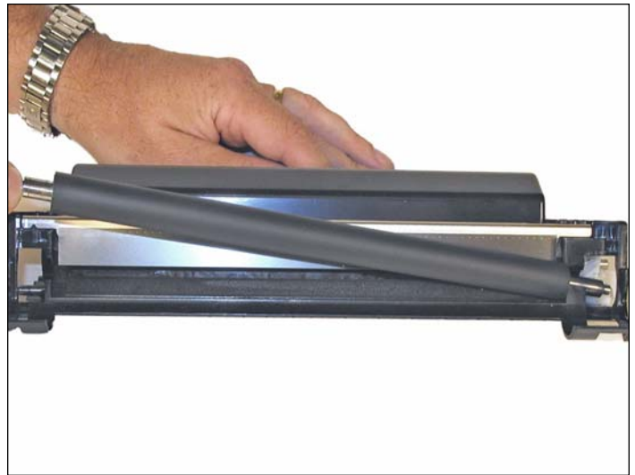
18. Clean and install the developer roller, long shaft side to gear side first.
