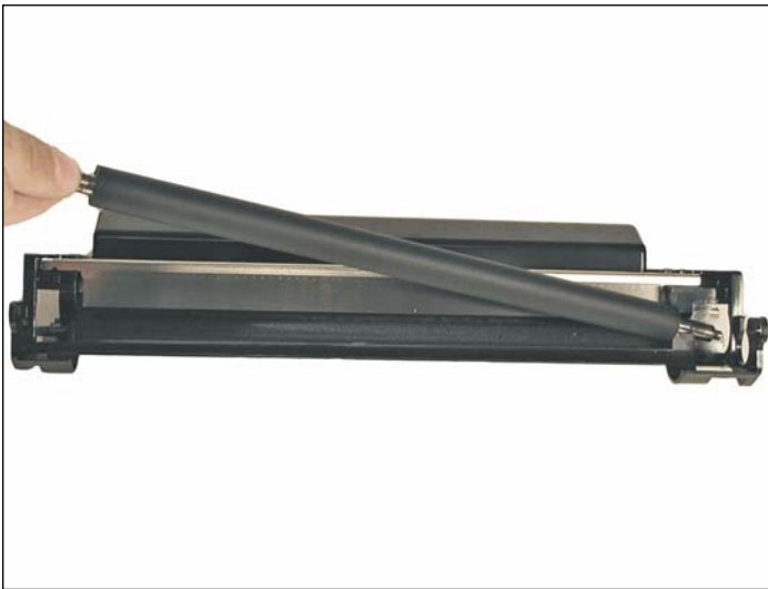
13. Remove the developer roller.
