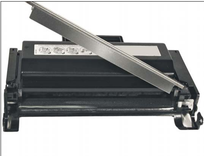
15. Carefully pry up the doctor blade.
