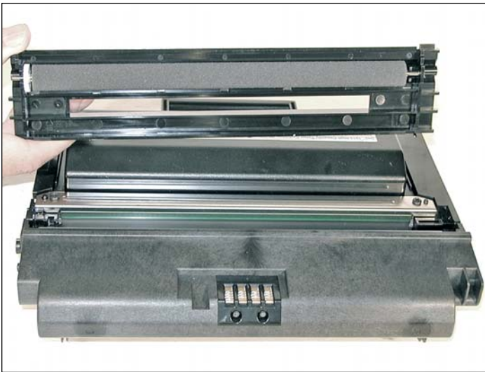
7. Lift off the roller assembly.
