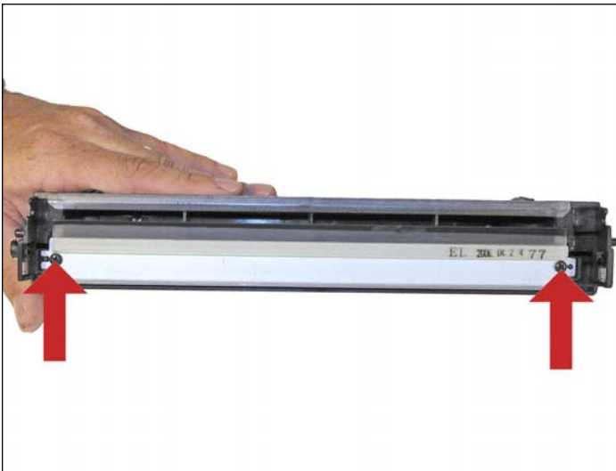
26. Remove the two screws and the wiper blade. Clean out all the toner from the hopper.
