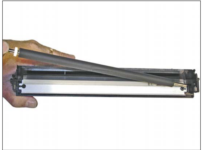
25. Slide the PCR to the non-contact side.
