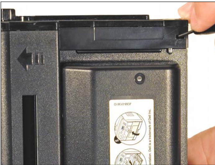
3. On the top edge of the end cap, there is a plastic tab.
