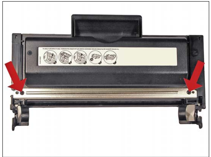
14. Remove the two screws on the doctor blade.
