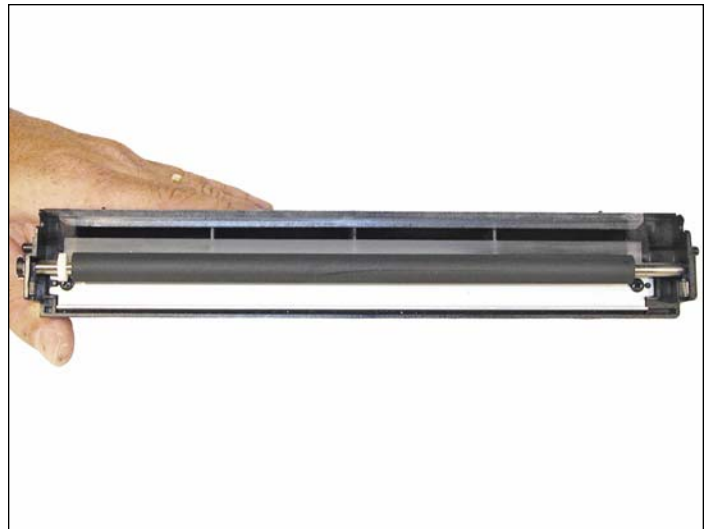
29. Install the PCR by sliding the long shaft side through the non-contact side. Bring it back to fit into the contact side.
