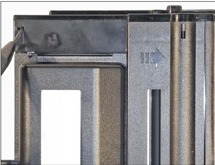
6. On the top edge of the end cap, there is a plastic tab.
