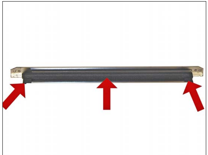
16. Clean the doctor blade and foam seals. It is too early to say exactly what chemical to use on the blade, but so far 99% isopropyl alcohol seems to work.
