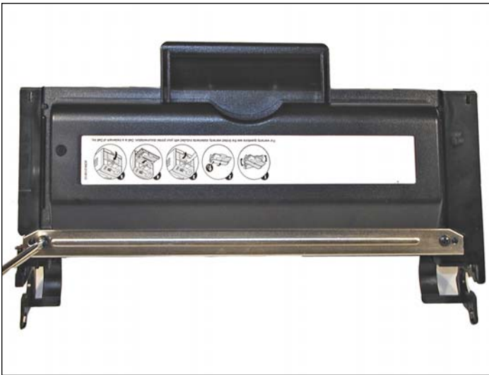
17. Replace the doctor blade and two screws.
