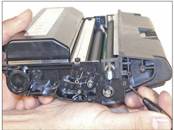
8. Carefully pry up the side plastic piece to release the waste chamber.
