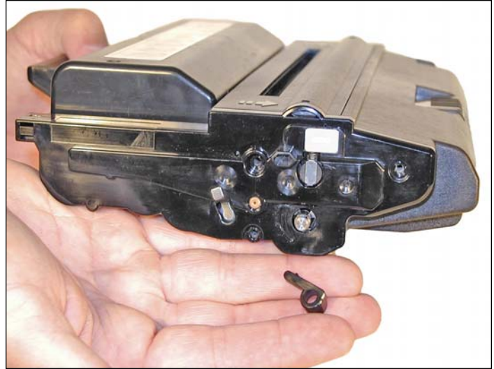
2. Gently pry off plastic drum axle bushing. Keep this bushing with the appropriate end cap when removed. Each side is different.
