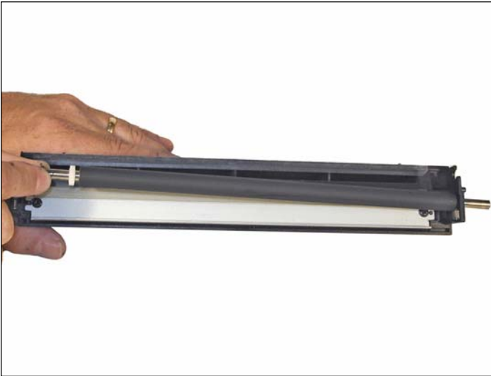
25. Slide the PCR to the non-contact side.
