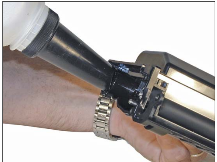
21. Fill the hopper with appropriate amount of toner for use in ML-3050. Check for leaks.
