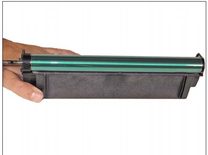
23. Slide the drum axle out from the side opposite the E-ring.
