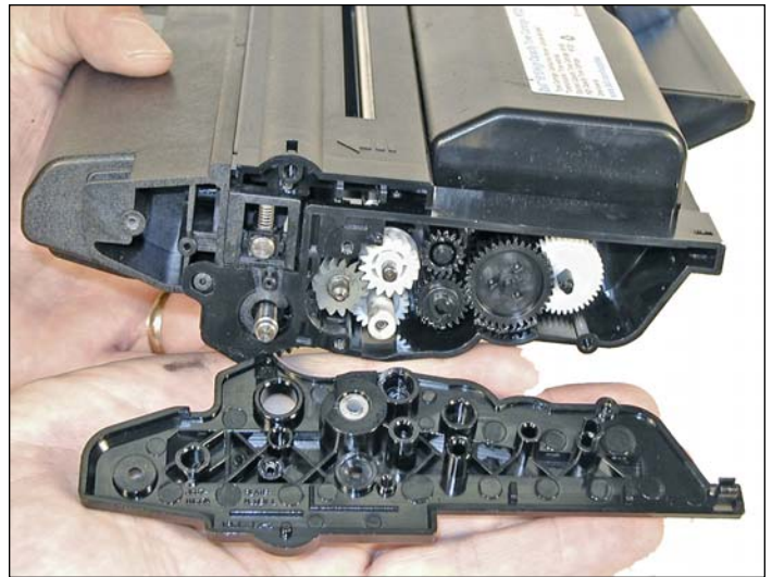
6. On the top edge of the end cap, there is a plastic tab.
