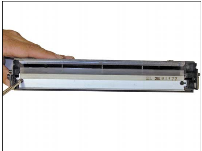
27. Coat the new wiper blade with your preferred lubricant.
