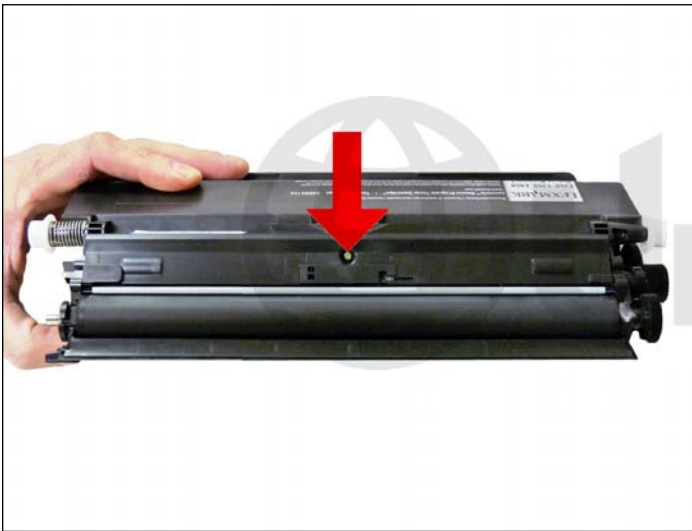
19. Re-install the developer roller cover and screw.
