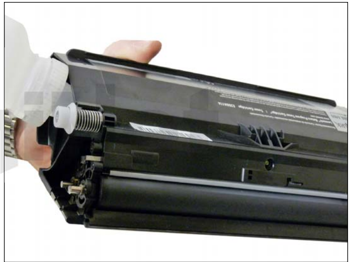
20. Fill the cartridge with the proper amount of toner for E260/360/460/X264/363/364 and install the fill plug.
