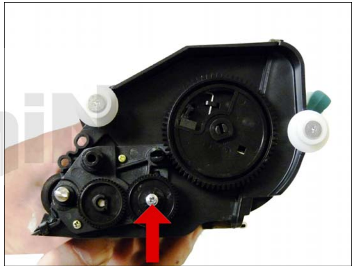
9. Remove the screw and lower idler gear.
