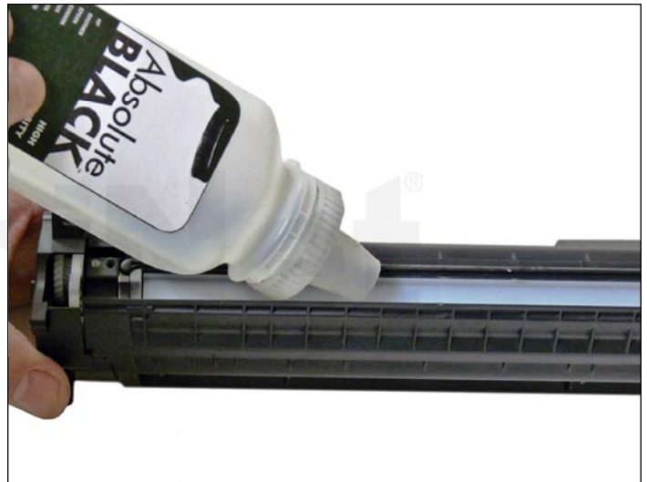
30. Fill through the magnetic roller opening with 120g of toner for use in P2035 "A" cartridge, or 290g for the "X". There is no fill plug in these cartridges.
