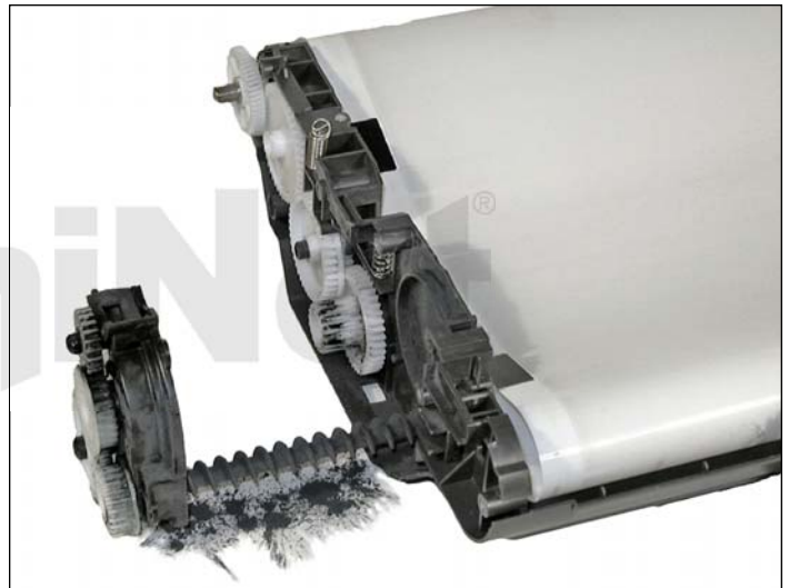
18. Pry off the black cover and gears. The cover is glued on. Take your time and work it off. Do not remove the gears from the cap!
