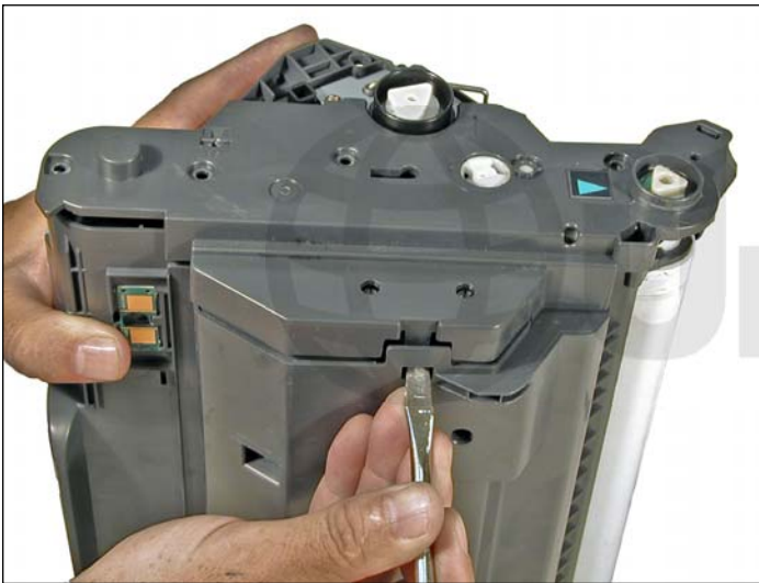
6. Press in on the bottom and top tabs to release.
