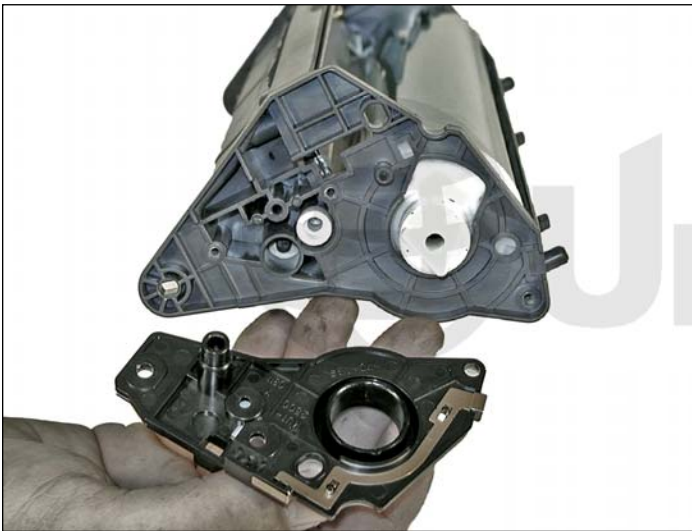
31. Press in on the copper contact, and remove the plate.
