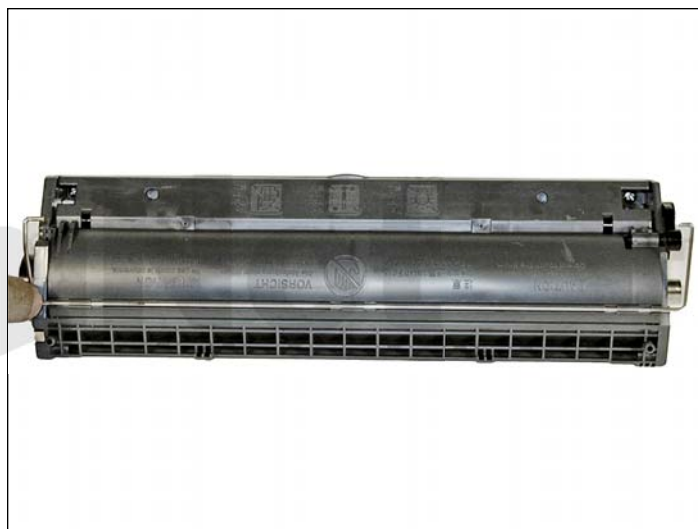
26. On the drum unit, remove the metal drum cover bars from the cartridge.
