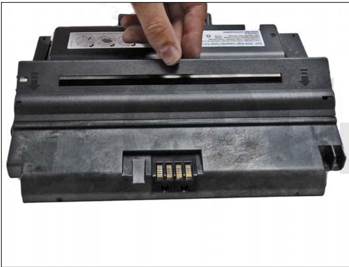
34. Install the roller cover assembly.
