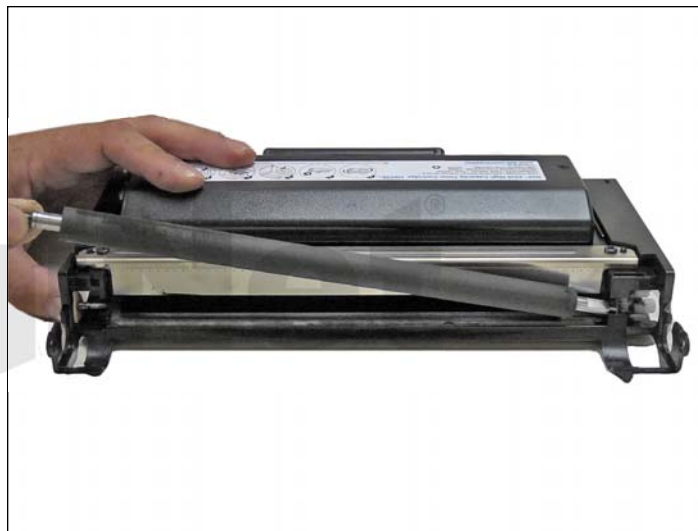
18. Clean and install the developer roller, long shaft side to gear side first.
