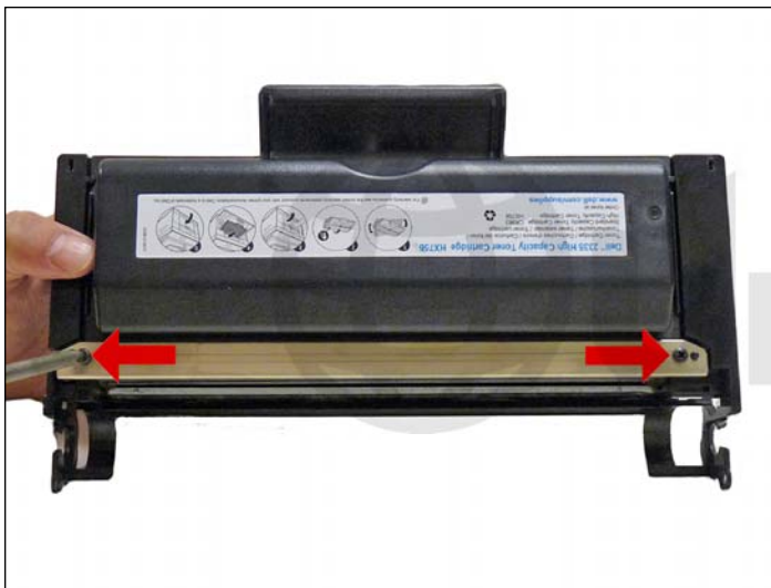
17. Replace the doctor blade and two screws.
