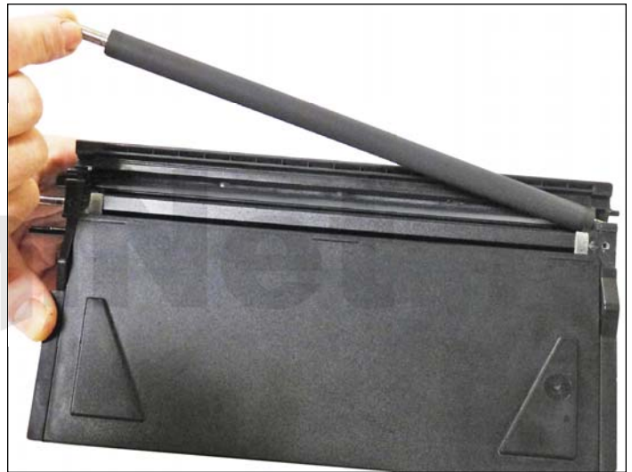
28. Remove the developer roller.
