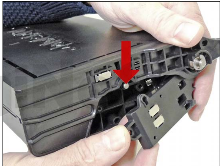
3. Carefully lift up on the contact plate to get access to the hinge pin (the contact plate cannot be removed yet).
