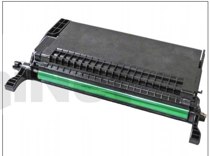
38. Place the two halves together.
