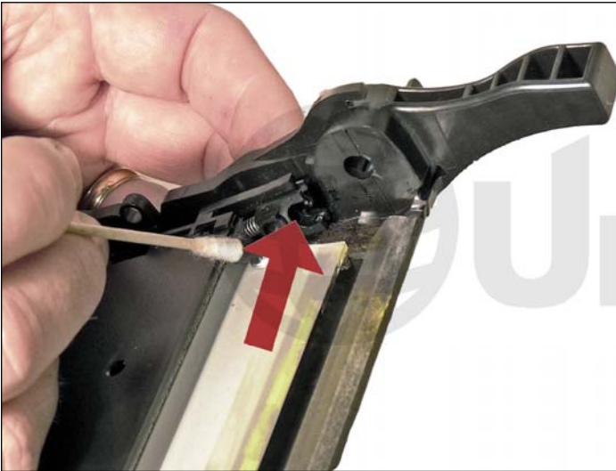
16. Place a small amount of conductive grease in each of the PCR holders, and on the PCR contact plate.
