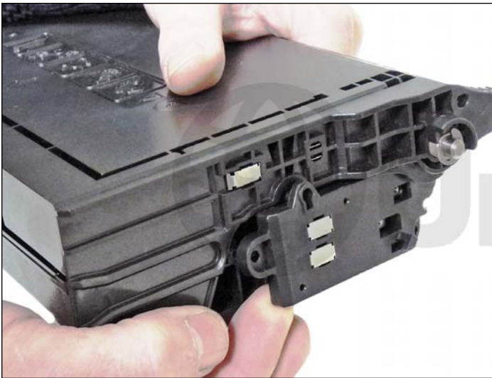
3. Carefully lift up on the contact plate to get access to the hinge pin (the contact plate cannot be removed yet).
