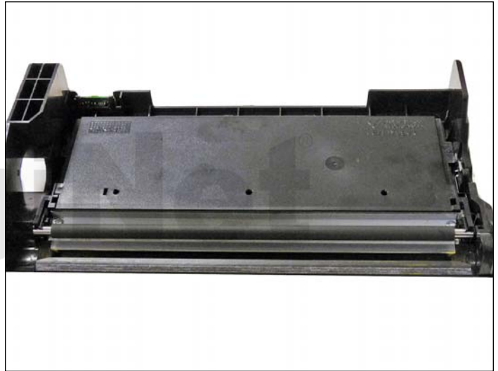
17. Install the cleaned PCR.
