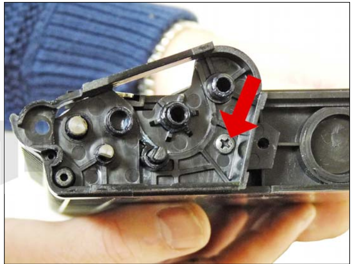
24. Remove the inner plastic gear plate and screw.
