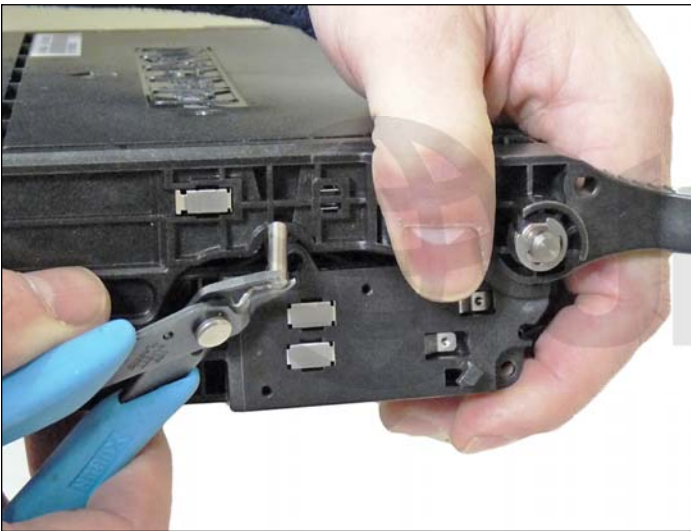
4. With a pair of wire cutters, remove the small hinge pin.
