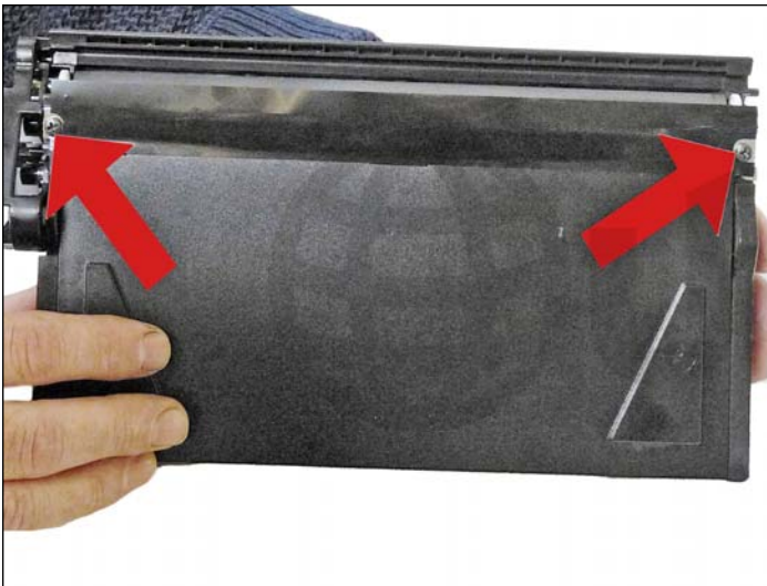
25. Remove the two screws on the doctor blade.
