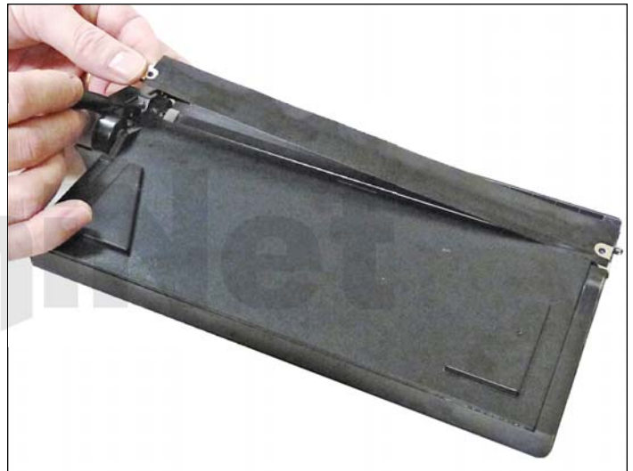
26. Carefully pry up on the doctor blade.
