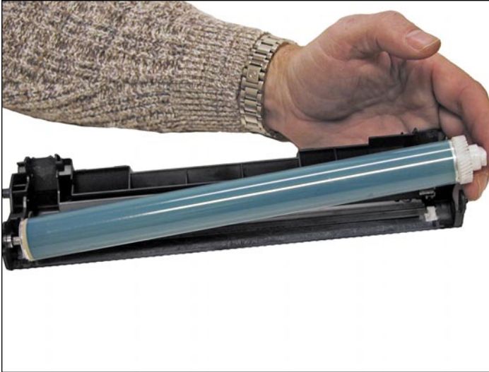
11. Install the new or cleaned drum, hub side first.
