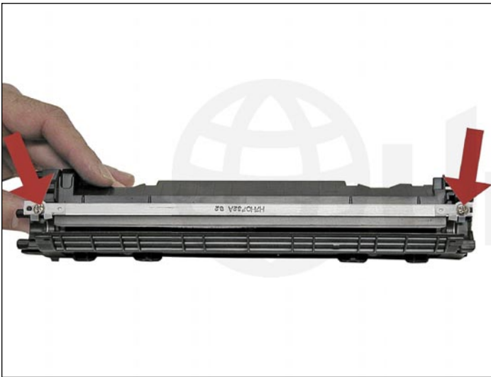
16. Remove the doctor blade and two screws.
