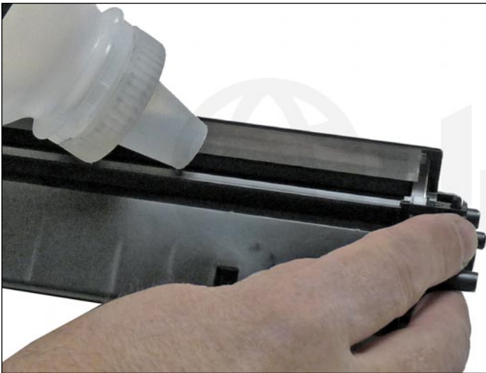
18. Fill the hopper with the appropriate amount of toner for use in the Canon 128.
